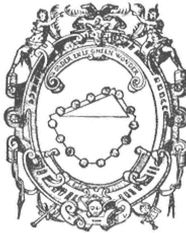
Figure 1 The vignette devised by Simon Stevin to illustrate his derivation of the law of the inclined plane
